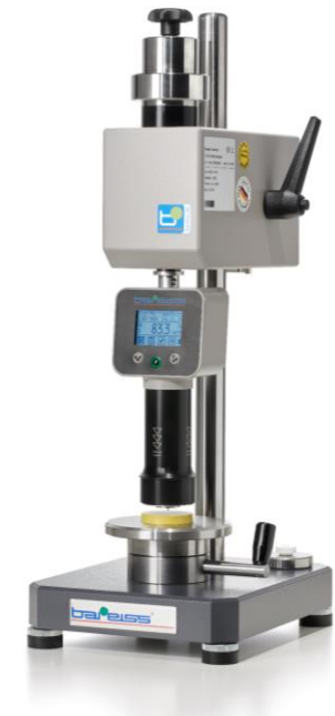
Test Stand BSA Automatic test stand with lowering speed of 3.2 mm/s acc. standards
